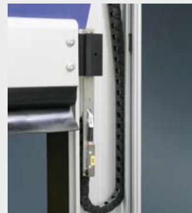
Integrated cable chain guides cables for pre-running photocell or electrical safety contact edge inside the side frame.
