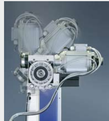
Drive unit position can be chosen in steps of 45°.
